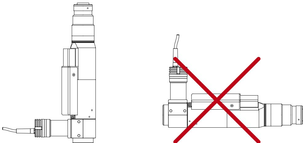
MZMT12X series lenses must be operated according to the drawing above.
